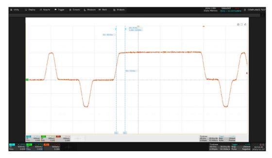
Figure 6-9 Details for Overshoot Test Waveform
