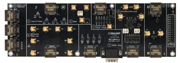
Figure 3-1 Ethernet Electrical Compliance Test Fixture Board
